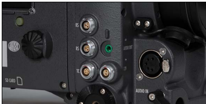
Figure 10: 24 V outputs (RS) and 12 V output
