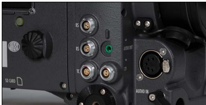
Figure 24: Connectors on right side
