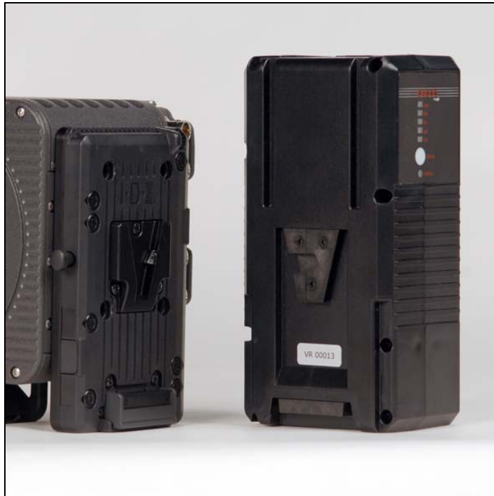
Figure 8: ALEXA with BAB-V and V-Mount battery
