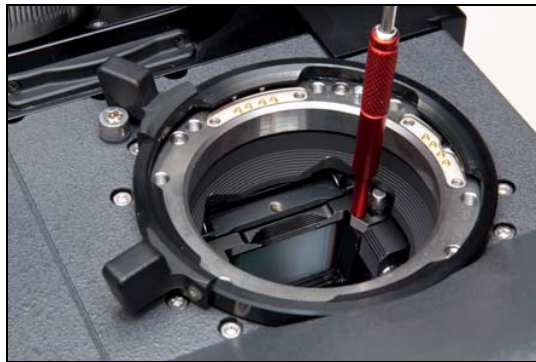
Figure 102: Ground glass in camera with Ground Glass Puller attached
